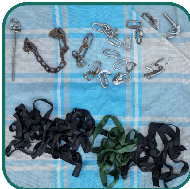
Above: Collection of anchors replaced in Davis Creek.
